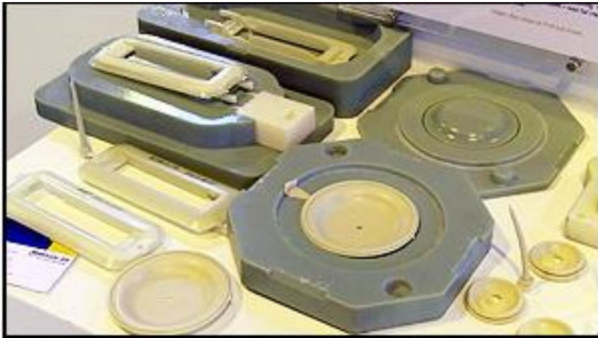
3D printed injection molds and patterns
