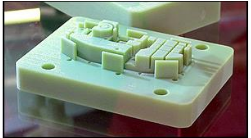
3D printed injection molds and patterns
